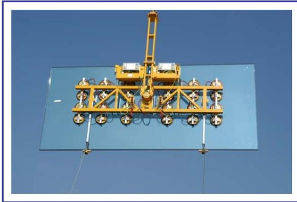
The Glas Zange company expanded its necessary machinery with a further vacuum lifting device for the tower glazing from us. A Kombi Akku-Device 7211-CeDe with maximum carrying capacity of 1200 kg was ordered for turning through +/- 90°. Additional adjustable supporting feet at the device secure the transport for such extreme glass superstructures like the insulating glasses used for the tower glazing without a risk of shifting the insulating glass structure.
