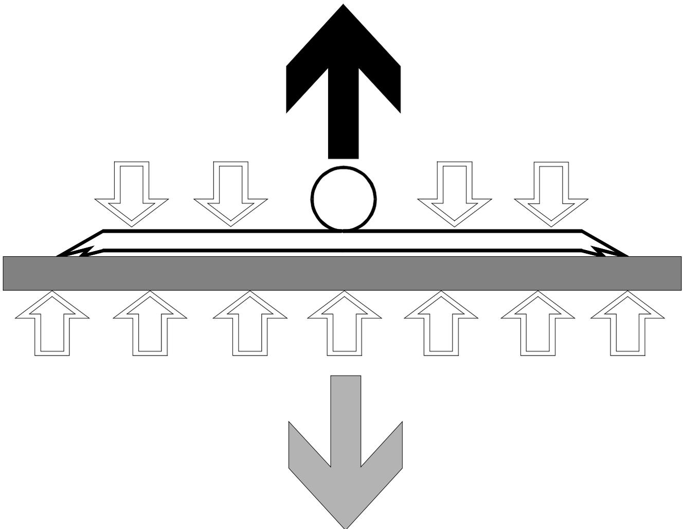
The retaining force is calculated as follows:  $\text{Product} = \text{surface} \times \text{pressure differential}$ . If this value is exceeded the suction cup pulls-off and this is called the pull-off power.
