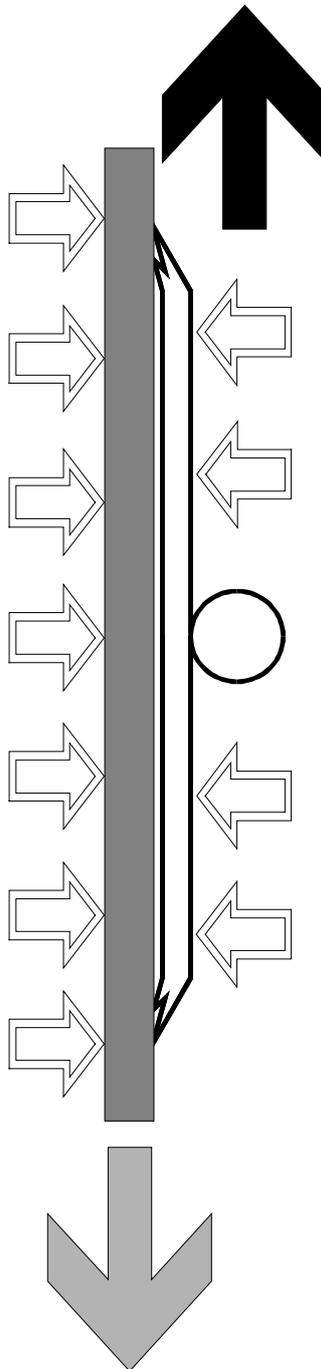
In general, the retention force is essentially lower in a vertical direction than in a horizontal one. If this retention force is exceeded, the suction cups slip off slowly. This is called the slipping off force.
