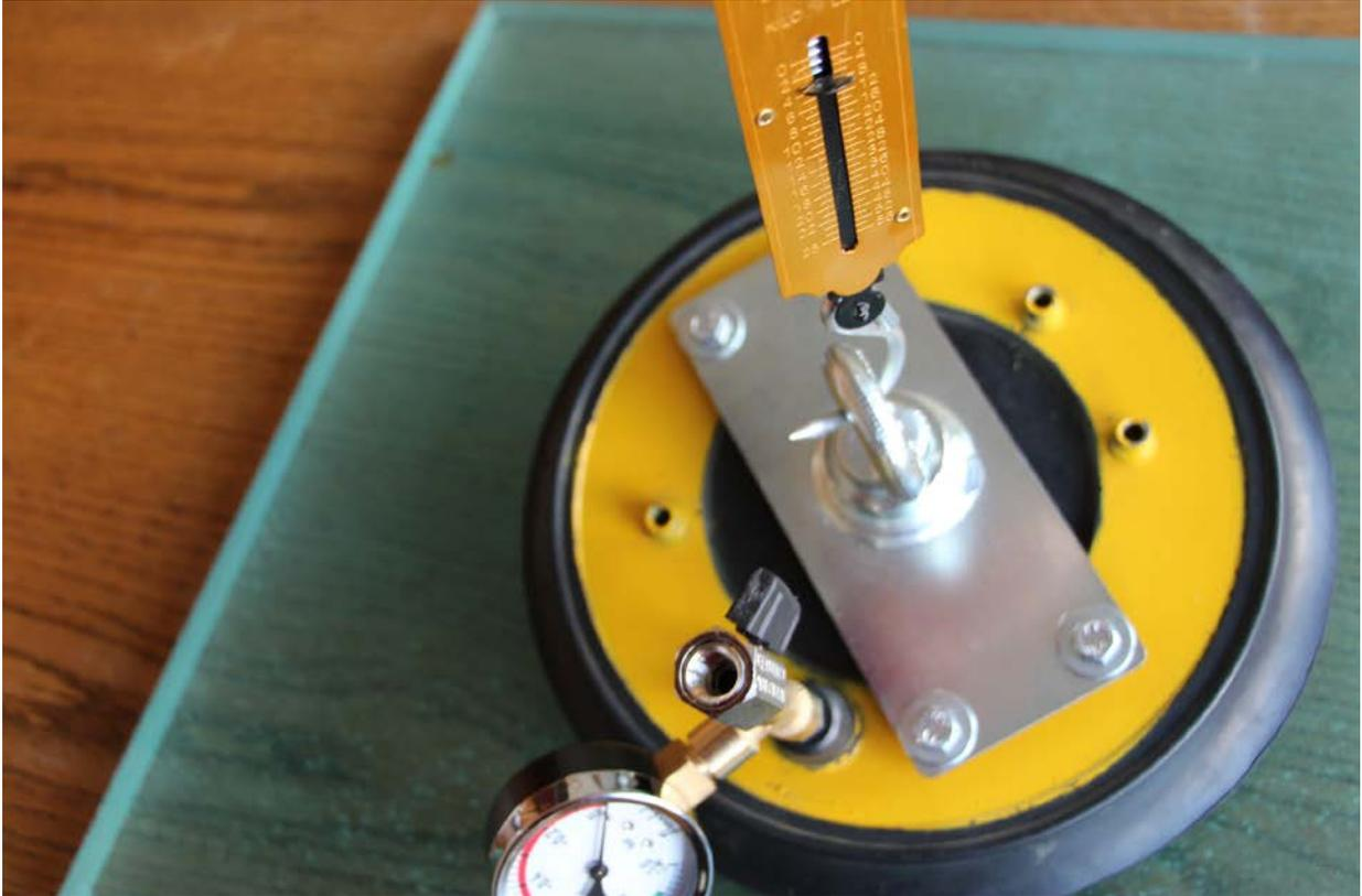
Place a suction cup with closed vent valve (no pressure applied) on a glass surface and move it around.
