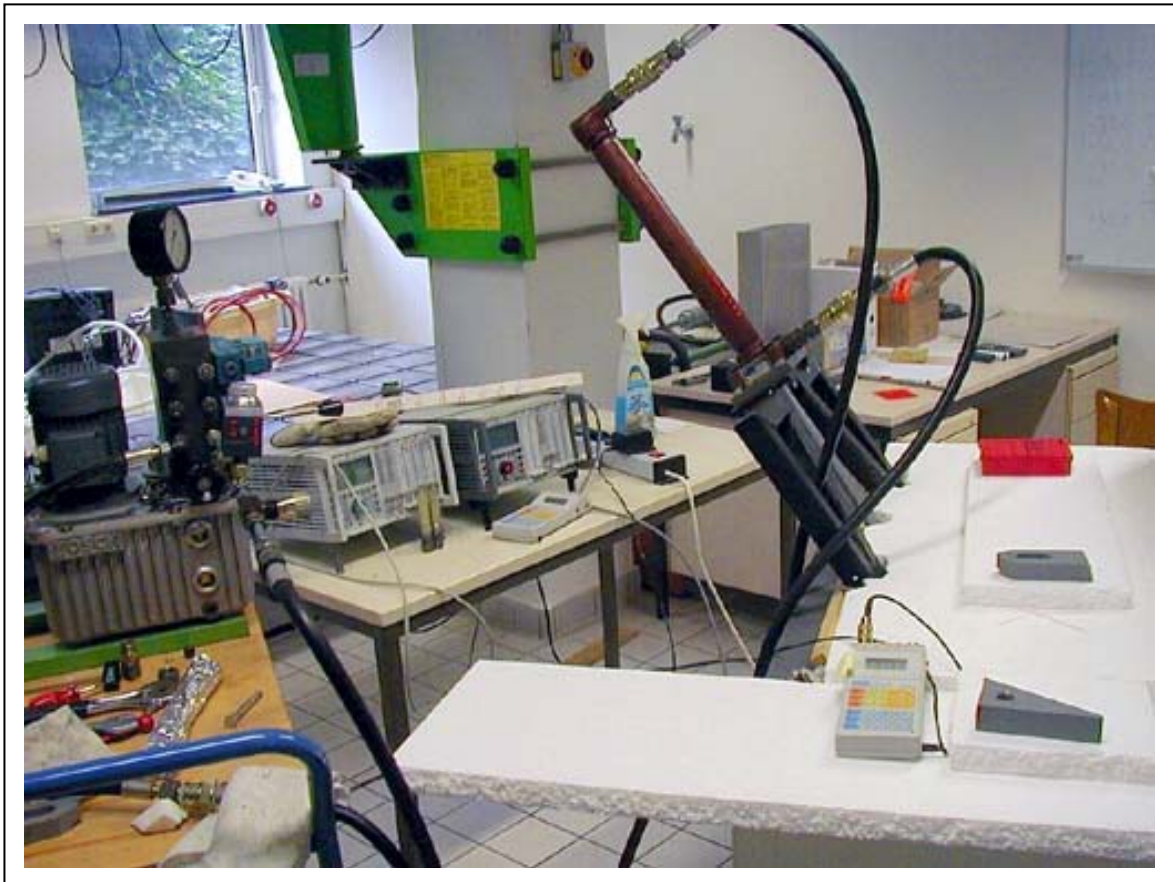
The photo shows the situation during the tension test, in front of the temperature display for the measuring point on the suction cup.
