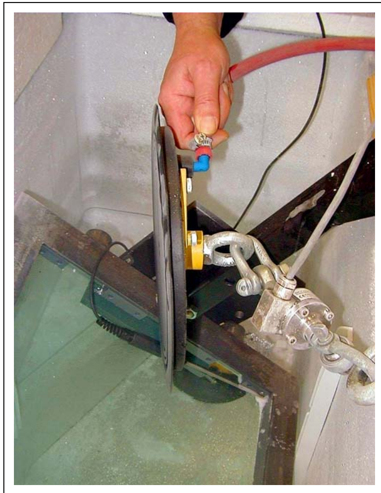
The photo shows at -30,8^{\circ}\text{C} the suction cup is stiff and not operative.
