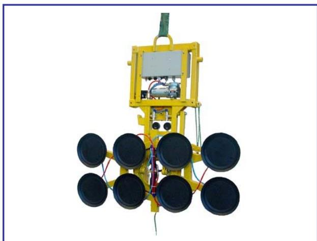
The device's suspension point has been brought that close to the loaded device's centre of gravity, that the loaded device's angle of inclination is very small, i.e. almost vertical, even at 1000 kg. This is very important when working between scaffolding and house wall.
