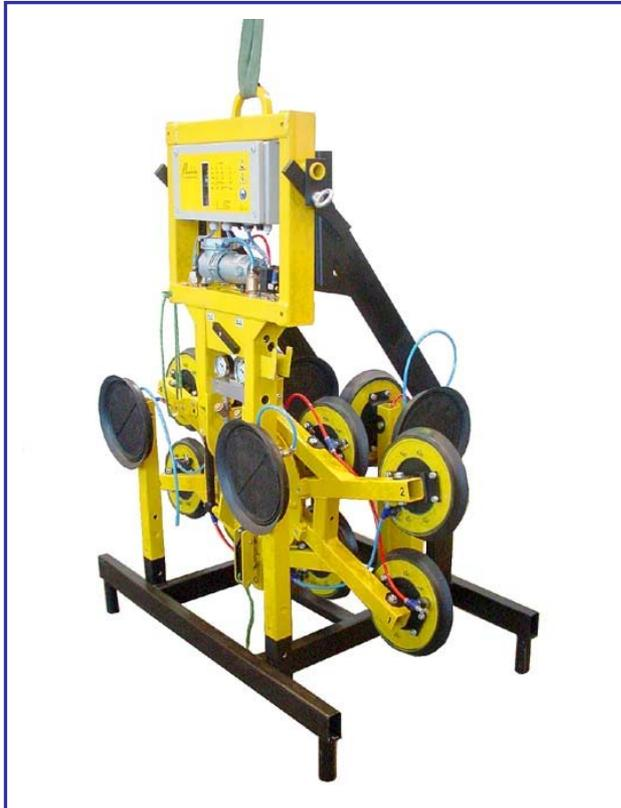
A transport frame to store and transport the **Kombi 7211-DS3** is also offered. This frame accommodates all the essential device parts and has been designed for simple and fast working. It is even possible to carry out maintenance work while the device is mounted on this frame.
