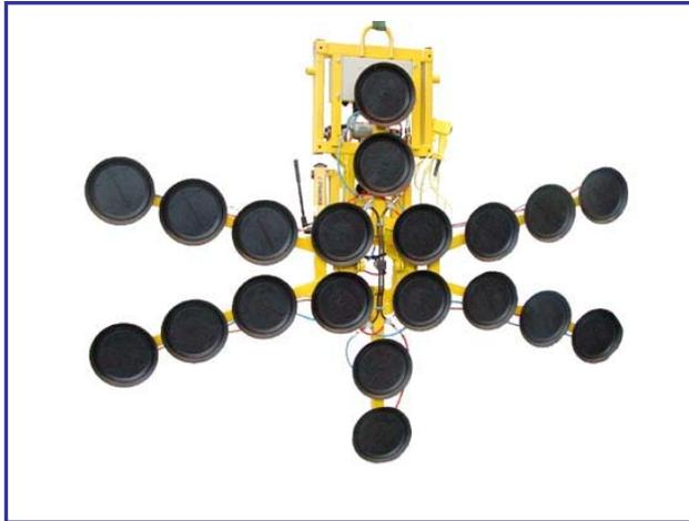
According to EN 13155 it is necessary for on-site operation that every vacuum circuit holds the rated load with twofold reliability. The **Kombi 7211-DS3** is equipped with differently coloured hoses, so that it is easy to recognise each vacuum circuit. In the **Kombi 7211-DS3**'s highest extension stage, each of its vacuum circuits is able to hold the test load of 2000 kg.
