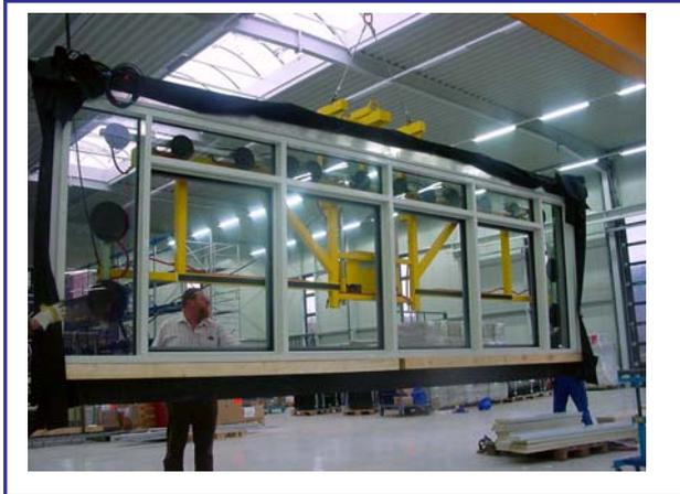
The specially chosen suspension point means that it is possible to transport the elements almost vertically. This was made a little more difficult by the roller shutters, but the solution won the client over. With the Kombi 7001-AB SO, the elements could be moved quickly and safely without any large change costs.
