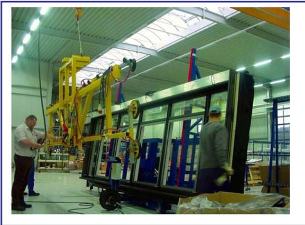
For the new internal medicine building of the clinic of the University of Würzburg, the company IGM from Medard got the task of delivering the facade elements. The full, pre-assembled, glazed window parts with a measuring up to 7.0 x 2.5 m are fitted with electric shutters.
