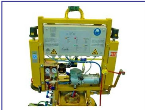
If we convert a 1-circuit vacuum lifting unit which we manufactured into a 2-circuit device, it receives a maximum of 8 suction cups and the load-bearing capacity is lowered to 400 kg on construction sites. Prior to any conversion, the device is subjected to a thorough test. After conversion, the vacuum lifting device is returned to the test stand and each vacuum circuit must be capable of bearing double the rated load in the form of steel plates.
