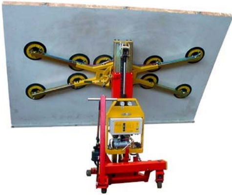
the maximum inclination depends on the height of stroke and the size of the transport load
