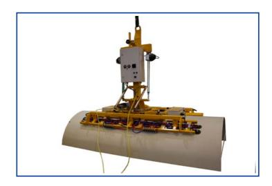
for planar stabilized, vertical lifting and transporting of convex and concave curved materials motorized tilting through up to 90 degrees motorized turning through ±360 degrees
